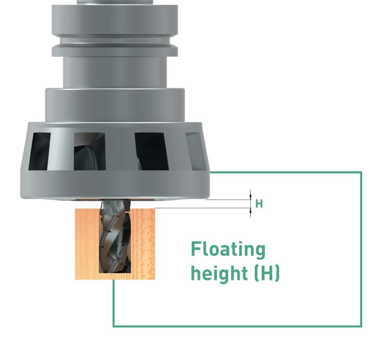
The use of Aerotech® at a floating height **(H) less than 2.0 - 3.0 mm** may reduce the air flow created and limit its capacity to remove dust.
